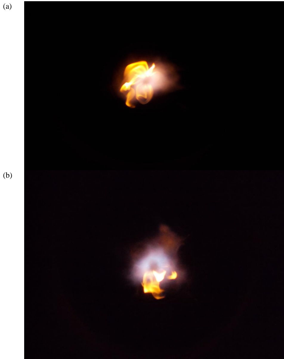
Figure 7: Flame image produced by (a) 45-30-Co-1.4 swirler, and (b) 30-45-Co-1.4 swirler
